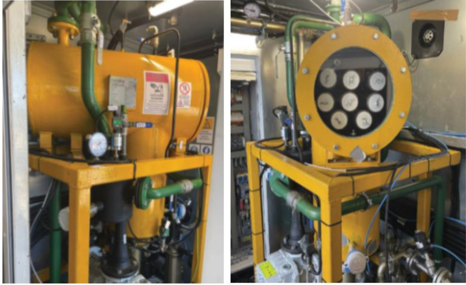
Vacuum Chamber consists of Coalescer Filters, Vacuum Pump & Booster for Removing Gas & Water from Oil
