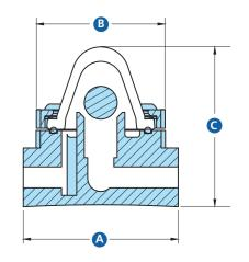
The Flow-Mon Rising Ball was developed to provide industry with a high standard in-line flow indicator to meet the requirements for a broad range of chemical, water, oil and gas applications. When calibrated flow indicators are not needed, the Rising Ball
